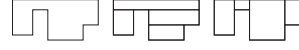
Figure 3 A shape to be formed (left) and the possible rectangle decompositions thereof (middle, right).
